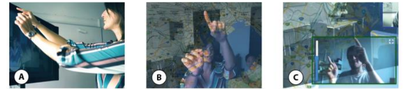
Figure 1: MirrorBlender is a malleable video-conferencing system that creates a WYSIWIS blended space for co-located and remote users. Deploying MirrorBlender in three hybrid meeting sessions, we studied A: deictic gestures, B: embodiment of mirror images, and C: how remote users are included and grab attention via their malleable representation in the interface.
